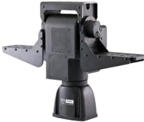
Figure 9 shows an image of a Pan Tilt unit. The unit can pan upto 360 degrees at speeds upto 300 degrees/second, and generally are provided with RS232 interfaces.
